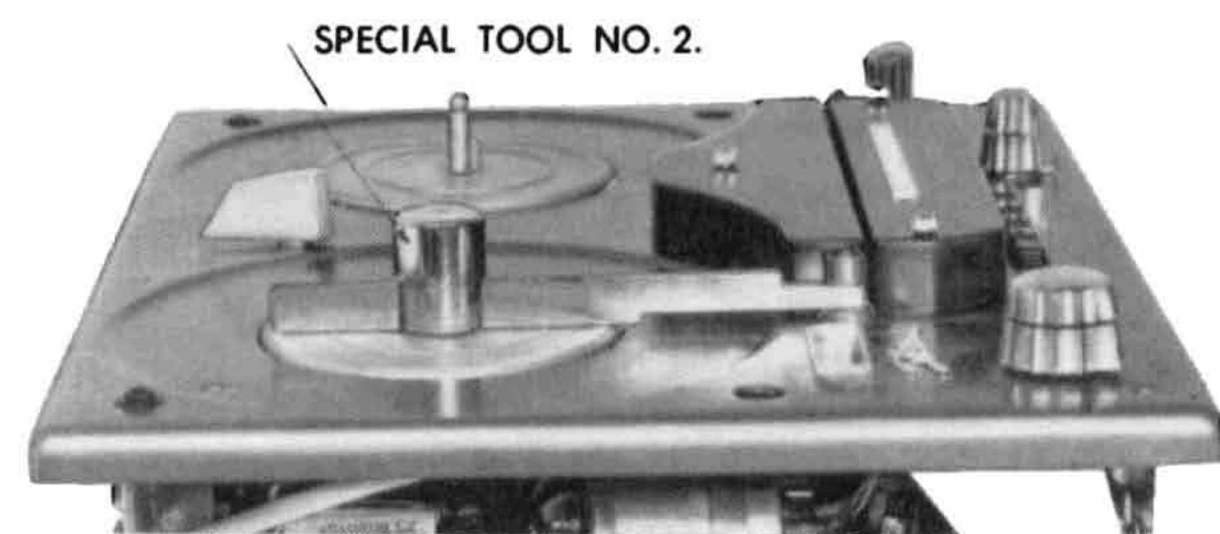
Fig. 19. Control of the horizontal position of the turntables with tool No. 2.
